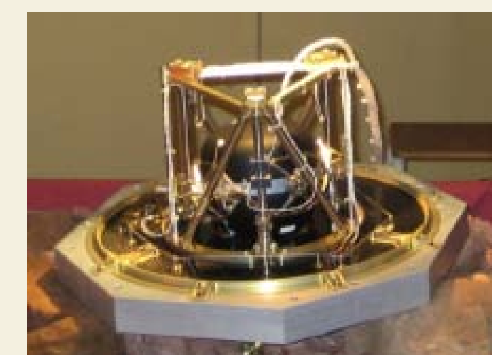
Fig. 3: Instrumented SPHERE on a Leveling (LVL) system prototype (courtesy MPS)
