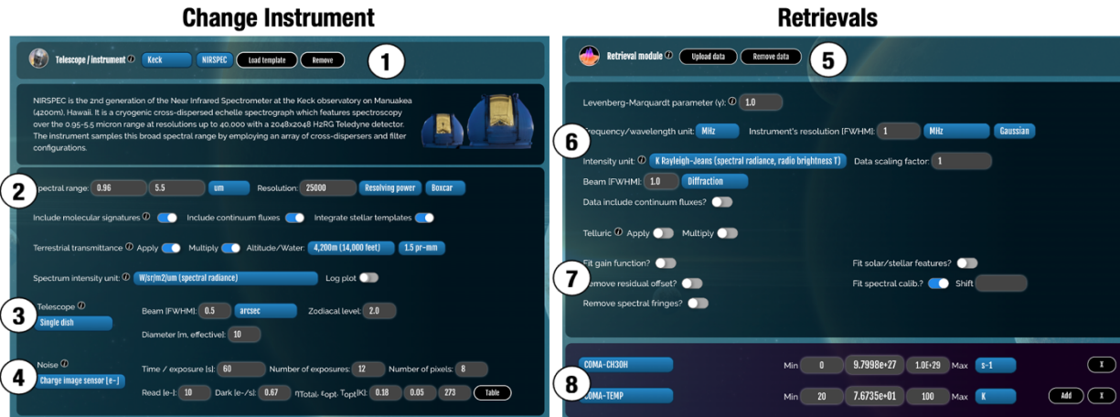
Figure 5: Website graphical user interface (GUI) for the instrument and retrieval sections. The different numbers indicate the main blocks within these interface windows.
