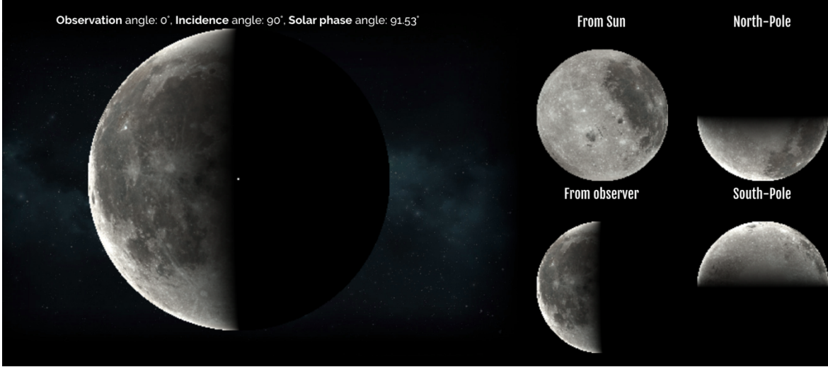
Figure 2: Lommel-Seeliger surface modeling of the Moon with PSG. The simulation was performed employing a constant phase function, P(G)=1 . The Lommel-Seeliger scattering model captures the quite homogeneous brightness observed on the Moon across the illuminated regions, while also models the significant brightening occurring at the illuminated limb.
