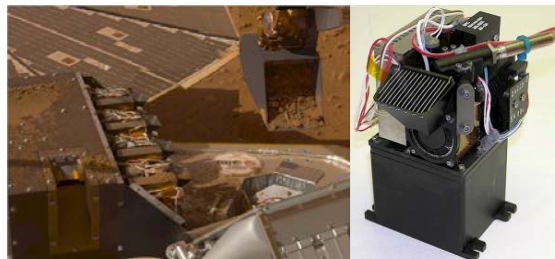
Figure 1. The Wet Chemistry Laboratory (WCL) as part of MECA (left) and a single WCL unit (right).
