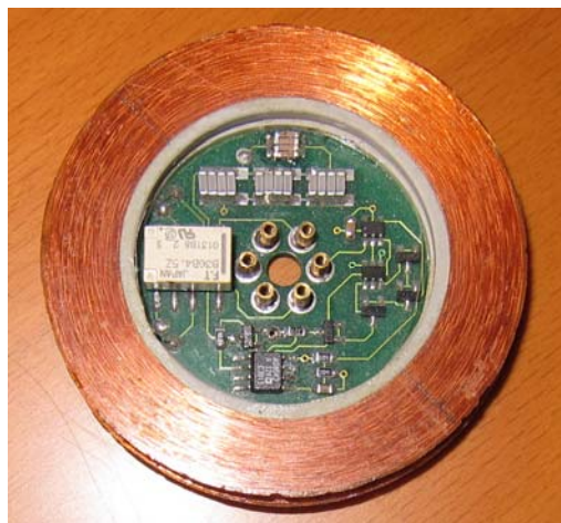
Fig 2. The sensor (coil) with control electronics of the commercial version SM-30 (ZH instruments) is currently being adapted for space applications as MSM (Magnetic Susceptibility Meter) instrument. The coil diameter is 5 cm.
