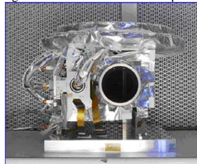
Figure 6 – The New Horizons Ralph telescope and detector assembly.
