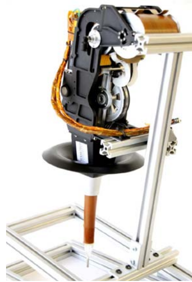
Figure 1. The latest prototype of the lunar heat flow probe with the stem stowed.
