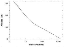
Pressure profile of the Titan moon measured by FMI's pressure sensor system (HASI-PPI) [1]
