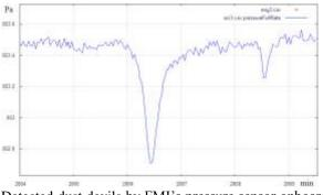
Detected dust devils by FMI's pressure sensor onboard Phoenix (MET-P)
