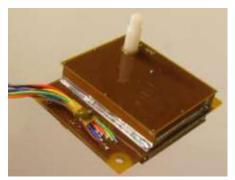
Pressure sensor unit "REMS-P" for Curiosity rover
