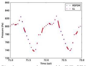
Diurnal pressure cycle measured by FMI's REMS-P pressure sensors onboard Curiosity rover. [3]
