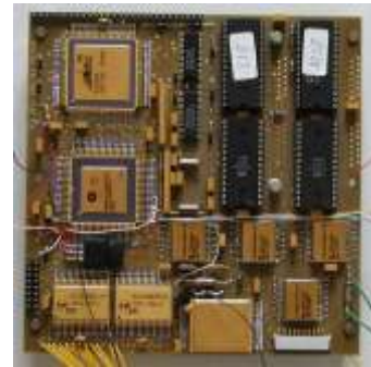
Fig-3: ICA and LAP DPU board
