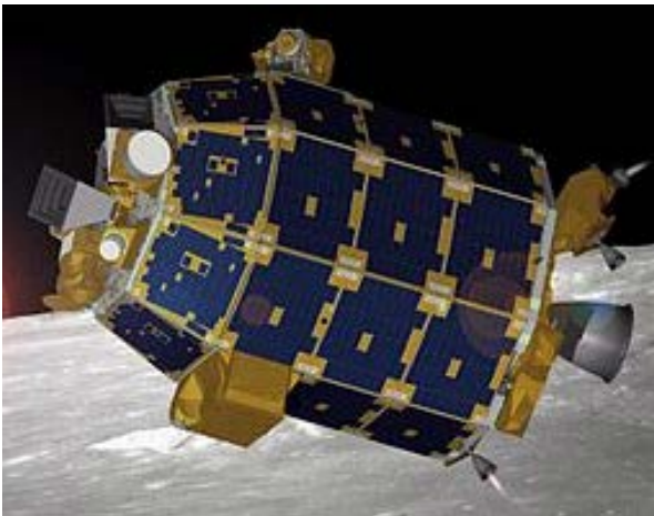
Figure 1. Artist's representation of the LADEE spacecraft with its three instruments and an optical communication technology demonstration instrument.
