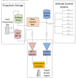
Fig. 4 – Pit-bot Propulsion System
