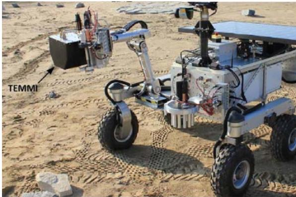
Fig. 1. TEMMI mounted on the arm of the Mars Exploration Science Rover (MESR) along with the Mini-Corer sampling tool (Mars Yard at the CSA in St. Hubert, Quebec).
