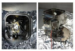
Fig. 2 MOMA-MS Engineering and Test Unit (ETU).
