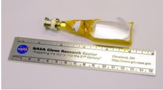
Figure 2 – Miniature scintillation/diode ionizing radiation detector as demonstrated.
