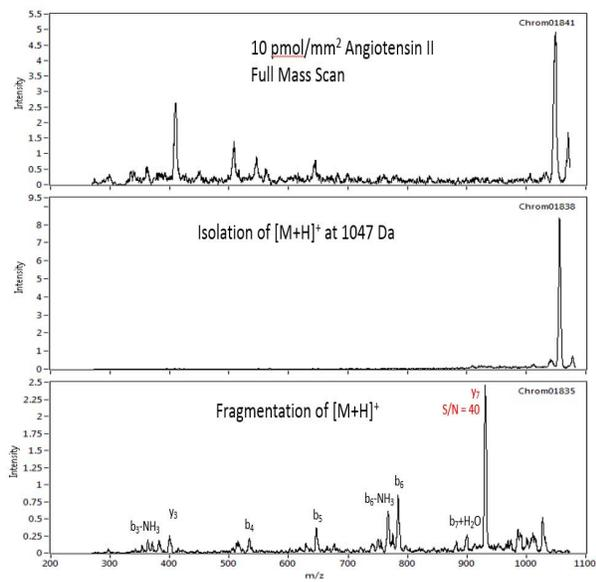
**Figure 4.** MS/MS operation demonstrated on 10 pmol/mm<sup>2</sup> Angiotensin-II ( $m/z$   $[M+H]^+ = 1047$  Da) in DHB matrix: (top) LDI-MS spectrum; (middle) Isolation of 1047 Da peak via SWIFT; (bottom) Fragmentation spectrum of the 1047 Da ion. MOMA-MS early prototype measurement.
