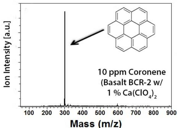
**Figure 2.** LDI mass spectrum of coronene ( $m/z = 300$  Da) doped at 10 ppm level in a Mars-relevant geological matrix (Columbia River Basalt - BCR-2) containing 1% perchlorate.
