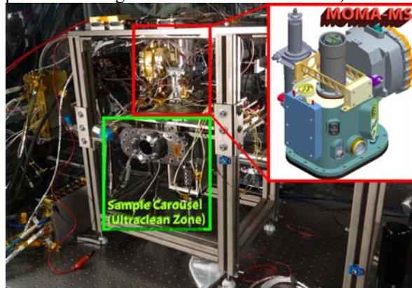
**Figure 1.** Engineering Test Unit at NASA GSFC, with inset illustrating MOMA-MS.
