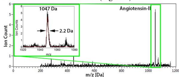
**Figure 3.** LDI mode mass spectrum of  $1 \text{ pmol/mm}^2$  Angiotensin-II ( $m/z [M+H]^+ = 1047$  Da) in DHB matrix. MOMA-MS ETU Measurement.
