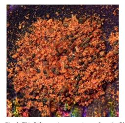
Fig. 3. This 2x2 mm microscope image from the Phoenix mission shows the mix of finer reddish particles, likely to dominate an airborne sample, and coarser gem-like polished grains that are transported by saltation and unlikely to be found in the air. The MOXIE images will be monochromatic.
