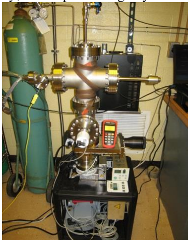
Fig 2- Characterization setup designed and built in house to test graphene sensor arrays
