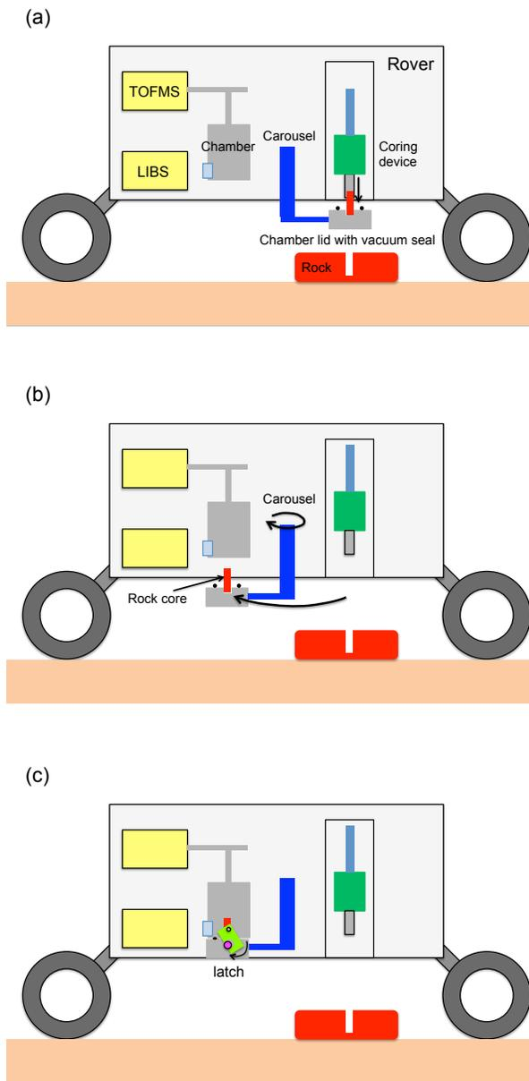
Fig. 3: Schematic diagram showing the sample delivery procedure. (a) A rock sample acquired by a coring device is transferred to a chamber lid. (b) A carousel delivers the rock core toward the position just below the sample chamber. (c) The rock core is inserted into the chamber as the lid elevates. A latch locks the chamber lid, producing a sealing force adequate to maintain vacuum.
