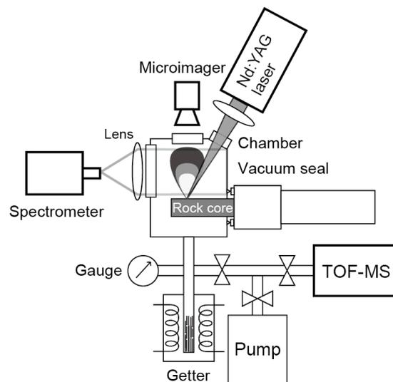
Fig. 1: Schematic diagram of a LIBS-TOFMS measurement. The concentrations of K and Ar are measured with LIBS and TOFMS, respectively.
