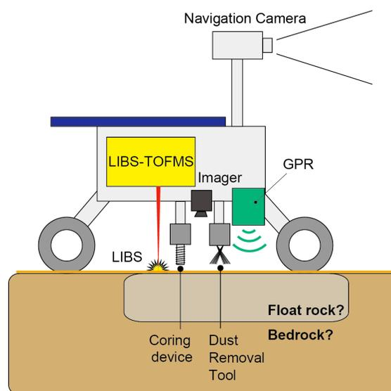
Fig. 2: Conceptual design of a rover equipped with the LIBS-TOFMS instrument, GPR, and the sample acquisition tools. GPR is used to check whether the rock is a part of bedrock or just a float stone.
