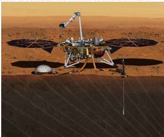
Figure 1 : InSight's lander on the surface of Mars, with SEIS on the left and HP<sup>3</sup> on the right
