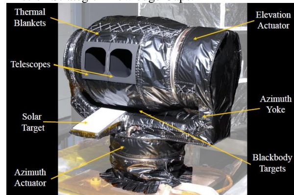
Figure 1: The MRO/MCS flight instrument during thermal vacuum testing at JPL.
