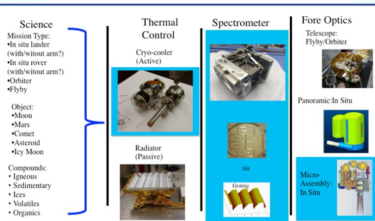
Items in blue boxes indicate hardware being integrated into instrument in the MatisSE program.
