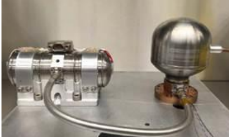
Fig. 3. Lockheed Martin cryocooler. This cryocooler is low mass (450 grams), has a long life expectancy (10 years) and has sufficient heat lift (500 mW heat lift at 77 K). It is well suited for integration with GeMini Plus
