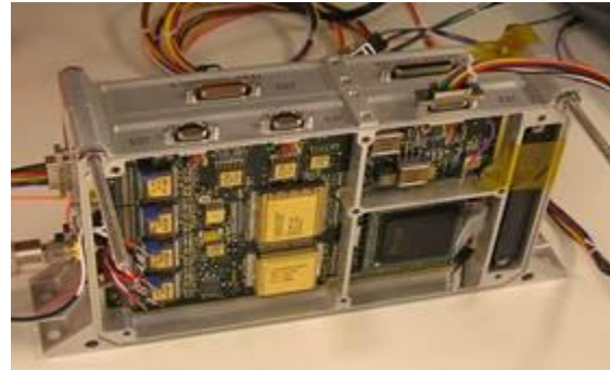
Fig 4. Digital Processing Unit (DPU) showing two “slices”.
