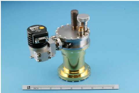
Fig. 1. GeMini Plus sensor housing including cryostat and miniature cryocooler. Not shown are power supplies and readout electronics.
