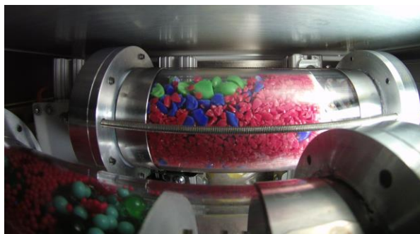
Figure 4: One of the first images downlinked from Strata-1. This image shows the angular, silica glass particles representing Experiment 2. Analysis is being performed now and results will be presented.
