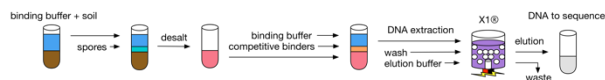
Figure 4: TRL4 nucleic acid extraction workflow and sample conditioning protocol for synthetic Mars analog soils.
