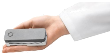
Figure 2: The MinION™ device is a nanopore sequencer that weighs less than 150 g, with a volume of less than 100 cm 3 .
