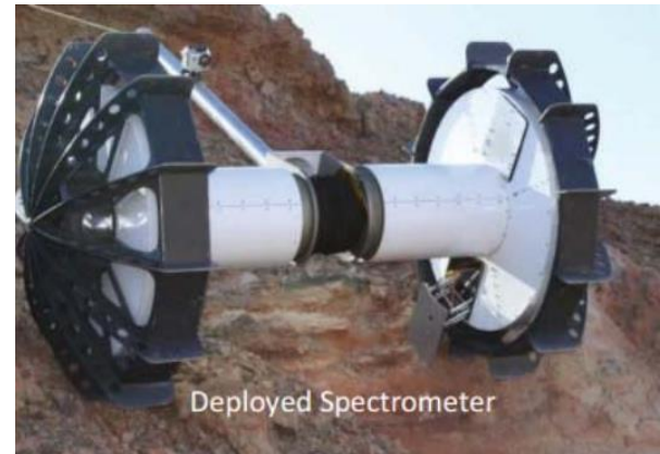
Figure 2. The Axel rover taking spectroscopic measurements on a slope of 40° (figure from [1]).
