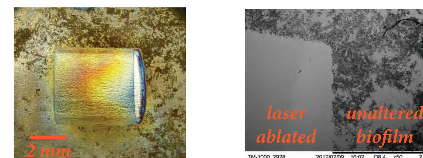
Figure 6: Laser ablation cleaning of a biofilm from 316 SS. A 4x6 mm area of biofilm was removed, scanning left to right. Left, visible image. Right, SEM image of removed edge.
