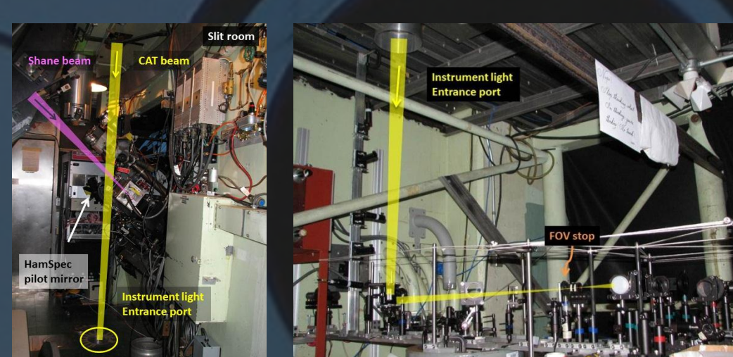
(left) 3m Shane telescope. (right) Light path through CAT outside the dome.
