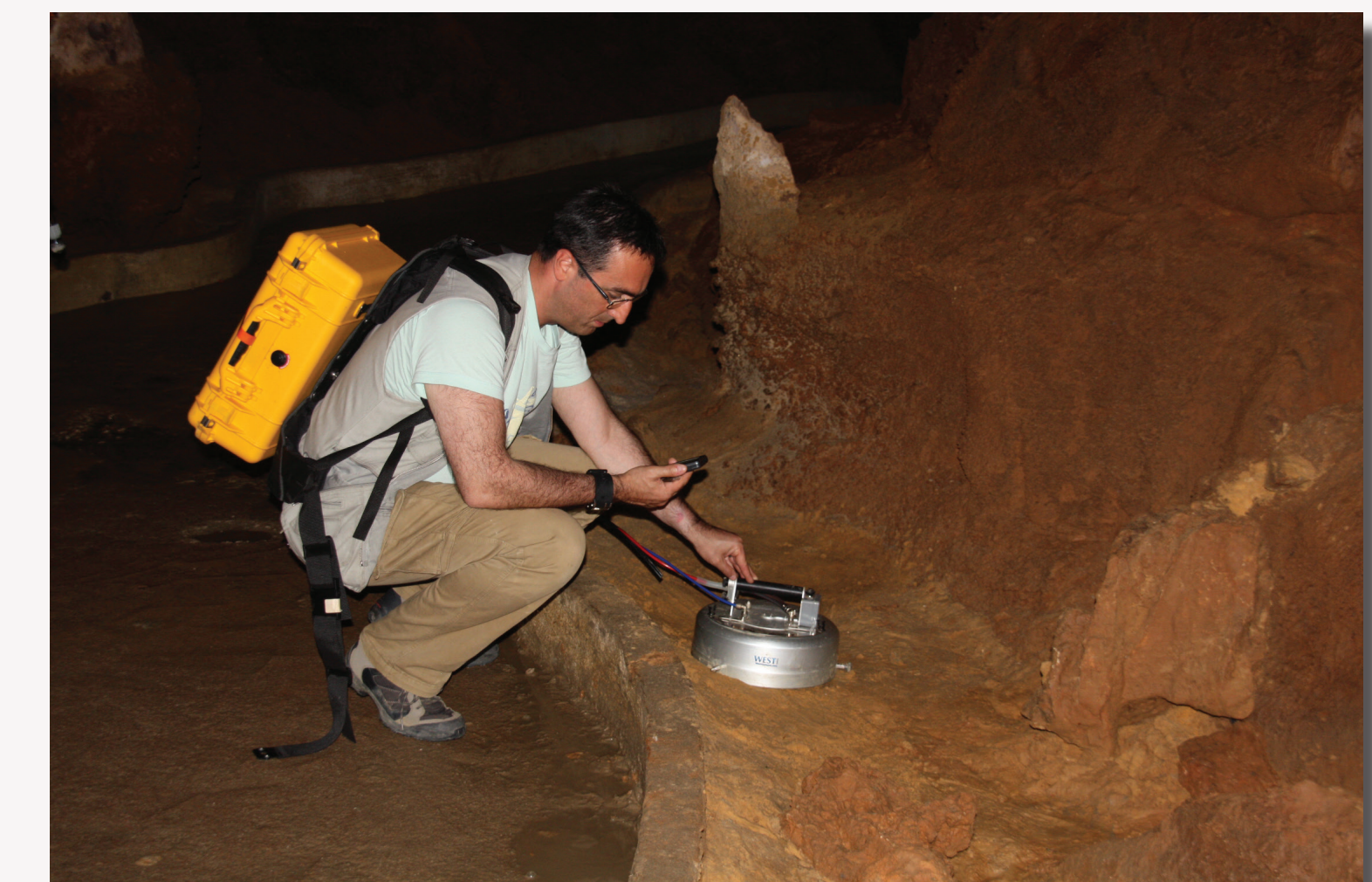
Figure 4: The WEST systems instrument measuring the flux of CH 4 in Diamond Caverns
