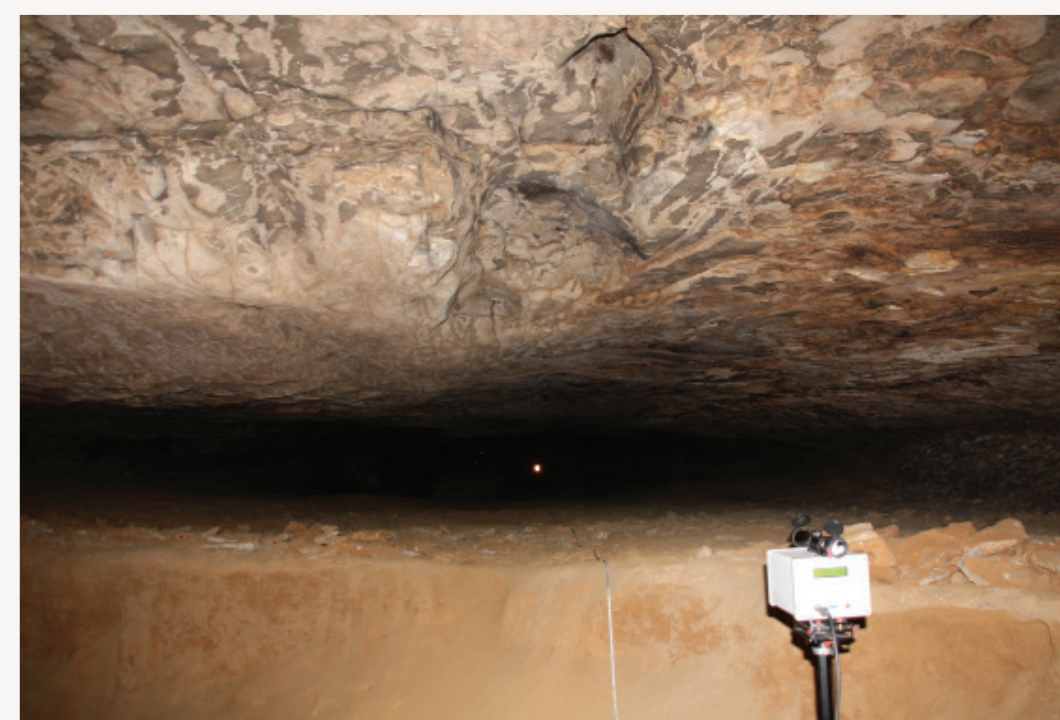
Figure 2: Deployment of the open-path laser (OPL) in a room in Mammoth Cave
