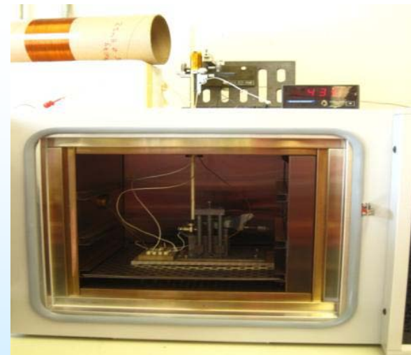
Photographs Of The Wireless Seismometer Sensor Test Setup.
