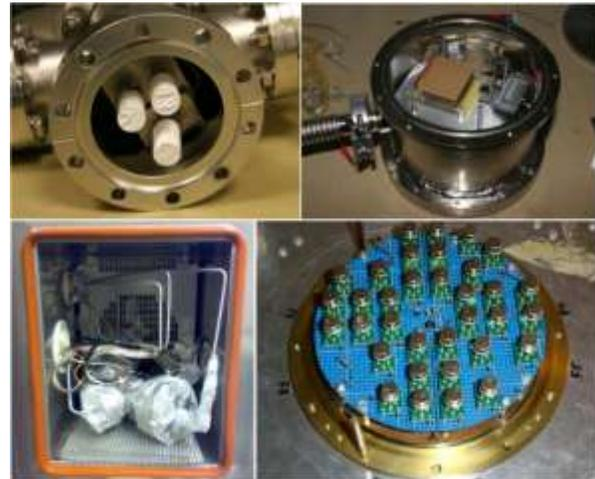
Various test set-ups of pressure and humidity sensors.
