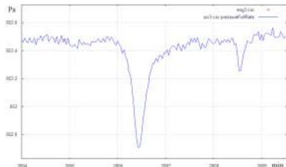
Detected dust devils by FMI's pressure sensor onboard Phoenix (MET-P)
