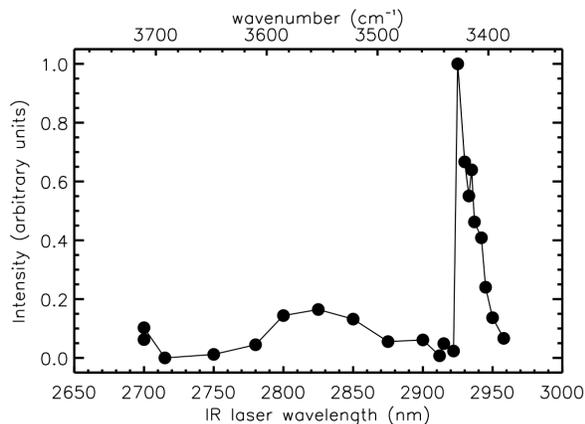
**Figure 3:** The dependence of the organic detection of the primary tryptophan fragment (130 Da) with IR desorption laser wavelength. The detection of tryptophan is optimized at a desorption laser wavelength of 2.925  $\mu\text{m}$ , corresponding to the tryptophan NH vibrational absorption feature. A broader secondary peak from 2.75 – 2.85  $\mu\text{m}$  corresponds to the broad  $\text{H}_2\text{O}$  hydration feature in epsomite.
