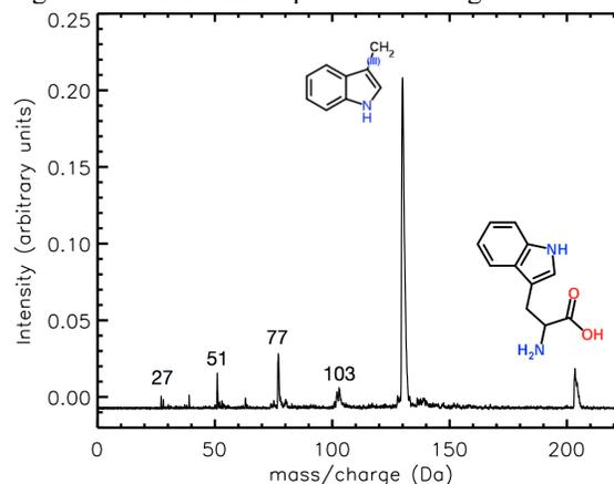
**Figure 2:** A mass spectrum of the epsomite sample doped with 0.1 wt% tryptophan collected by the L2MS with a desorption laser wavelength of 2.925  $\mu m$ . The major tryptophan fragment is located at 130 Da, and the parent peak is located at 204 Da.
