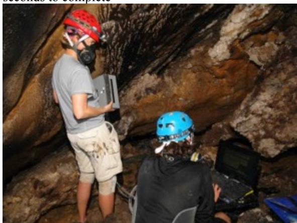
**Figure 2. PASA data acquisition in Cueva de Villa Luz in December 2013. Authors Chanover (left) and Uckert (right) are positioning the instrument and running the data acquisition software, respectively.**
