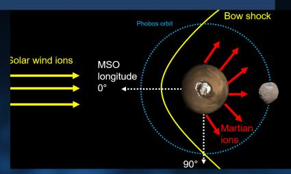
Phobos is bombarded by protons and alpha particles from the solar wind and by Martian atomic and molecular oxygen ions. 4 years of ion observations from MAVEN at the orbit of Phobos show that Martian ions  $O^+$  and  $O_2^+$  significantly sputter the surface of the moon.
