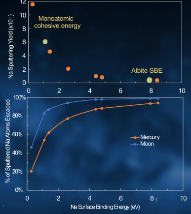
Results show Na SBE derived for albite is 30x higher than values previously used in sputter calculations, decreasing the yield by a factor of over 30! SBEs for minerals can be 8x higher than the monoelemental cohesive energy approximation often used to estimate compound SBEs.
