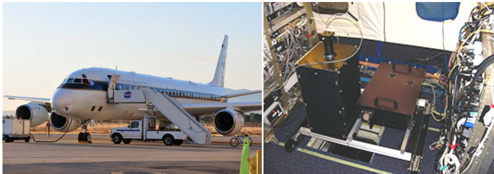
Fig. 4. (Color online) (left) NASA's DC-8 aircraft at DAOF prior to a methane flight and (right) the methane lidar in the aircraft. The lidar used two aircraft racks and a transceiver.
