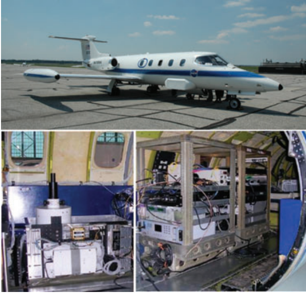
Fig. 2. Top panel: NASA Glenn Lear-25 aircraft. The nadir window assembly is just below the NASA logo. Bottom panels: photograph of the lidar installed on the aircraft showing the sensor head assembly (left-hand panel) and the dual aircraft racks (right-hand panel).
