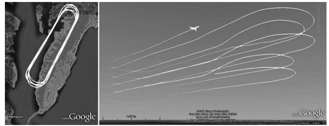
Fig. 6. (Left) Top view of the August 17, 2009, flight track (Chesapeake Bay close to Hampton, VA, USA): The same ground track (land and water) was passed five times in different flight altitudes (Source: Google Earth 2009). (Right) Side view of the flight track showing the five altitude levels (Source: Google Earth 2009).
