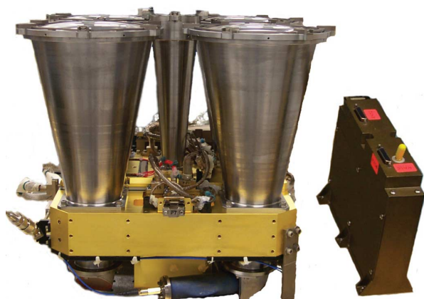
Fig. 14. Photograph of MLA at GSFC prior to delivery to MESSENGER [9]. The diameter of the four received telescopes is 14 cm.
