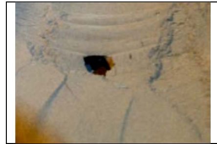
Figure 6- Regolith fails to maintain stability (creates a hole) when underlying surface has a hole. This effect does not occur if the regolith layer is thicker – due to more surrounding grains creating greater cohesion
