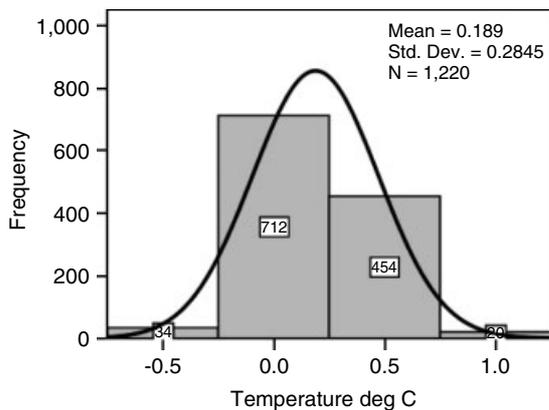
Figure 2. Temperature data frequencies (data points) as recorded by 61 ThermoChron iButtons in a 0.0 °C water bath
