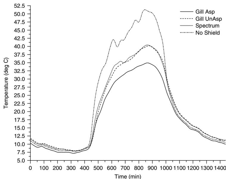
Figure 4. Temperature responses of Thermochron iButtons placed in a greenhouse setting employing different solar radiation shields (one without shielding). Although all iButtons responded to solar diurnal cycling, temperature response means between shields varied significantly ( $p < 0.05$ ). Graphs presented with 25-point smoothing
