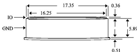
Figure 1. The dimensions (mm) of the Thermochron iButton are identical for the entire DS1921 family and others. IO: input/output. GRD: ground. A single data lead and ground is all that is needed for data transfer
