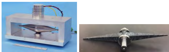
Figure 1: Left, rotor design, with 25 cm titanium rotor installed. Right, carbon-fiber rotor.
