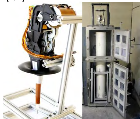
Figure 2. Heat flow probe penetrated compacted NU-LHT-2M simulant at 1 m/min. [4, 5]
