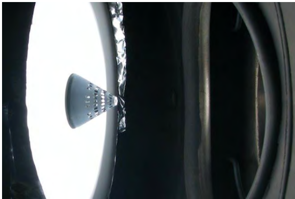
Figure 3: Solar balance testing of the MIPA entrance system. Illumination is from the right side. The white surface represents the HT-MLI.
