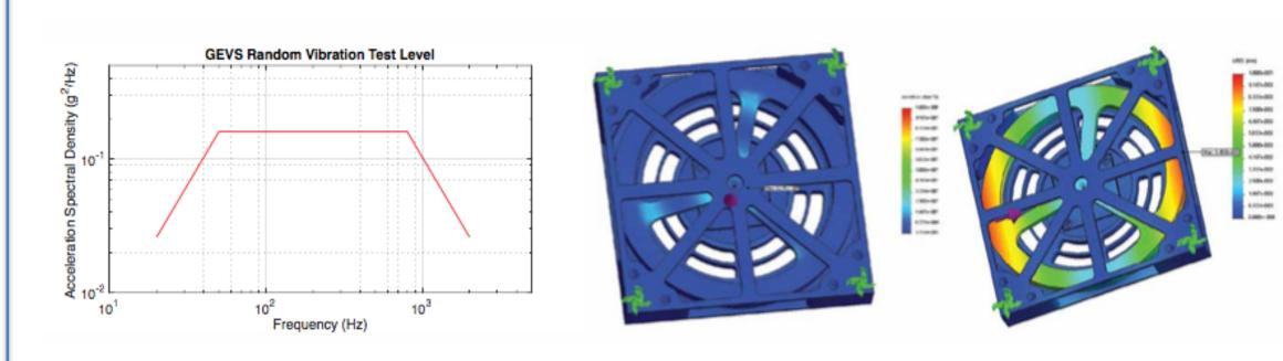
Simulation results for both the single axis and three axis designs, did not show significant differences in the load profiles. This analysis focuses on the shaft-mounted wheel since less is known about the mechanical strength of the outrunner design. The Table below shows the factors of safety derived from this analysis. Further testing under static conditions should be performed to determine the loads the motors can actually withstand.
