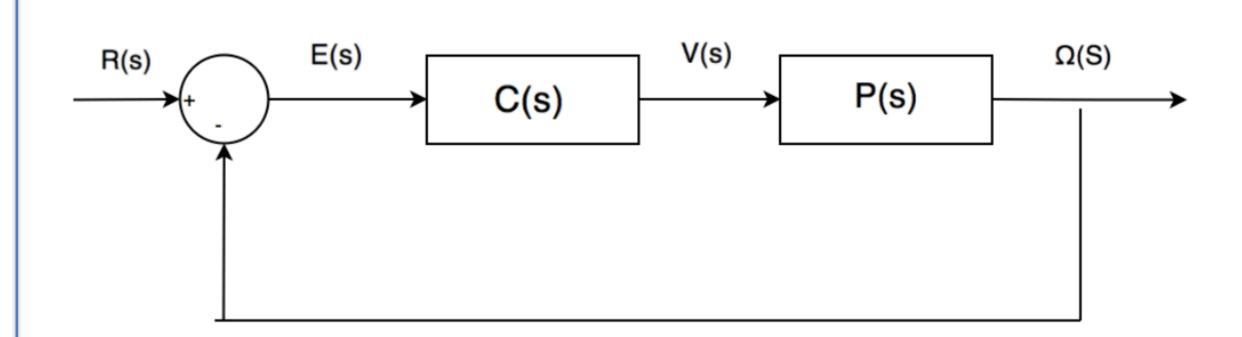
To test the robustness of our model, real-world factors such as a time delay and a discrete control cycle were simulated. In our system a discrete controller commands a motor controller with a slight electrical delay. We found that the altered responses only marginally deviated from the ideal system. The control cycle was short enough that continuous time models were considered valid.
