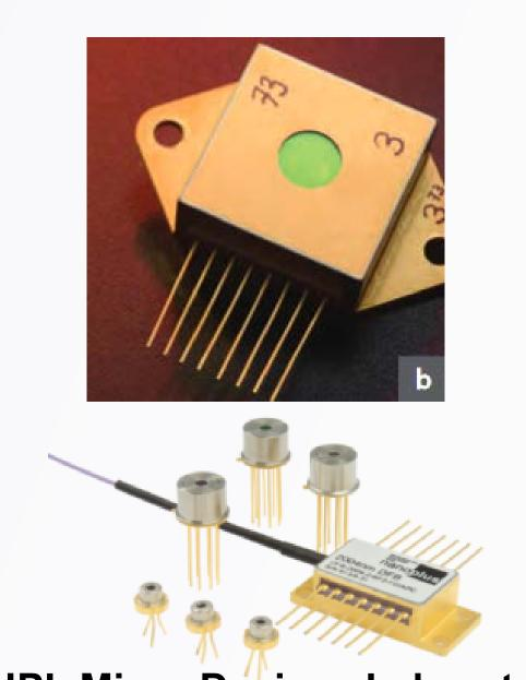
JPL Micro Devices Laboratory Interband Cascade Laser and Nanoplus Distributed Feedback laser used in the Tunable Laser Spectrometer on the Sample Analysis at Mars (SAM) Investigation. Webster, C.R. et al., 2015. Science 347 (6220).
